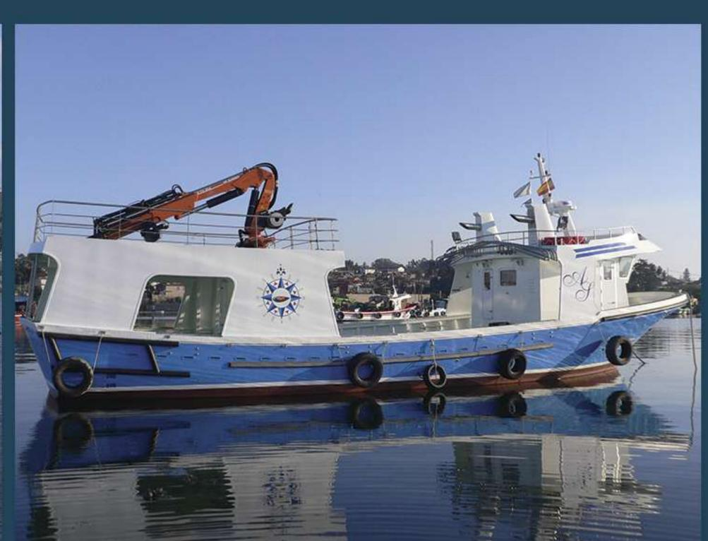
Designed according to the needs and preferences of each shipowner, these vessels are specifically adapted for work in mussel rafts, fish farms, and long-line culture. They have spacious, clear decks and high-capacity cranes. They are built with either conventional or single-use mold techniques, offering endless possibilities for dimensions and designs, in both monohulls and catamarans.
